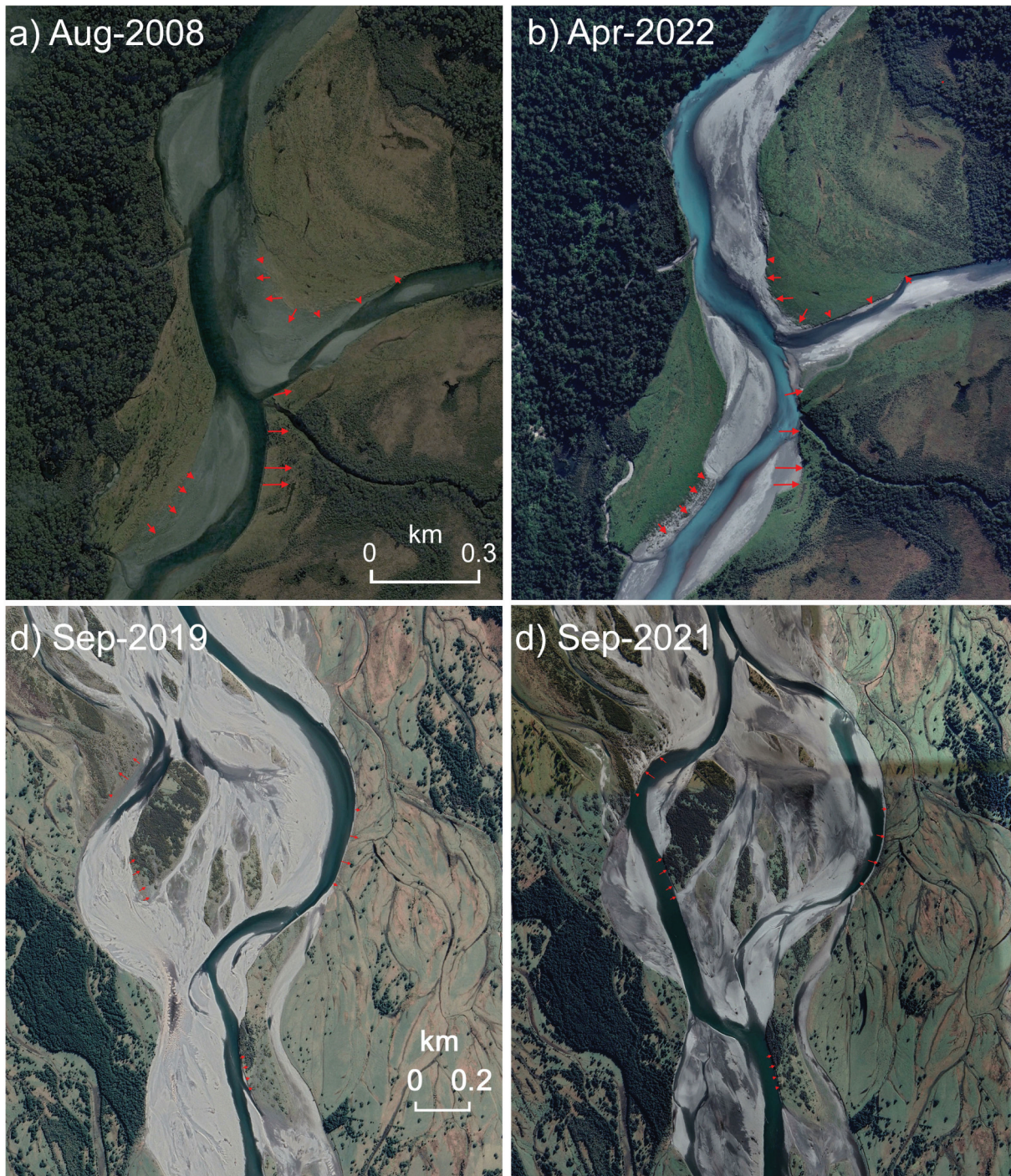
Figure 9. Channel migration, avulsion and bank erosion are challenges to maintaining permanent river runs in south Westland. a) Waitototo River in Aug-2008; b) Waitototo River in Apr-2022; c) Karangarua River in Sep-2019; and d) Karangarua River in Sep-2021.
